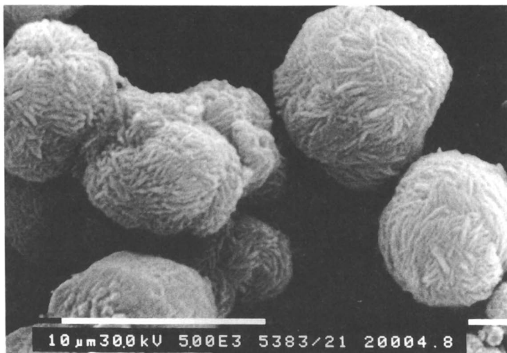
Figure 1: Bayerite with "woolball" morphology from ageing sodium aluminate solutions
